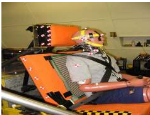
Pre-impact position of the rear impact dummy in the volunteer seating position
