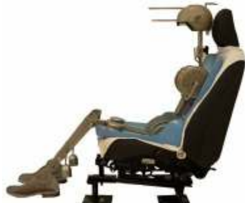
3-D H machine and HRMD used to measure head restraint height and backset in version 1 of the WG20 test procedure
