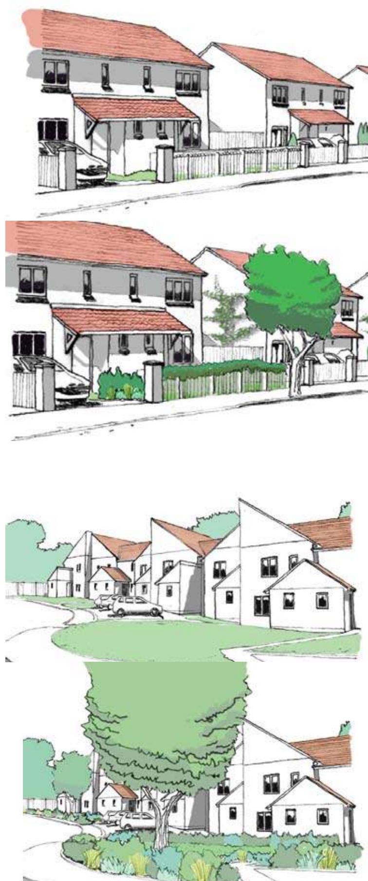
Fig 1: Two illustrations showing how a scheme can appear much more attractive with more mature soft landscaping (HATC / Jan Randall).
