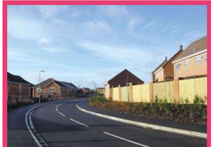
Fig 17: A road designed primarily to carry traffic. Not only is it a soulless place, but its value to pedestrians as a safe walking route is also undermined by a lack of surveillance from nearby houses (Tribal Consulting).
