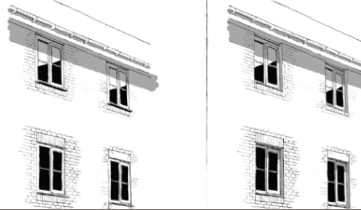
Fig 36: The elevation on the left is flat. The right one offers 'surface relief' by setting back the windows a little (HATC/Jan Randall).
