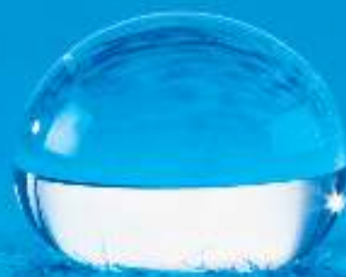
P2i's technology dramatically lowers a product's surface energy, so that when liquids come into contact with it, they form beads and simply run off
