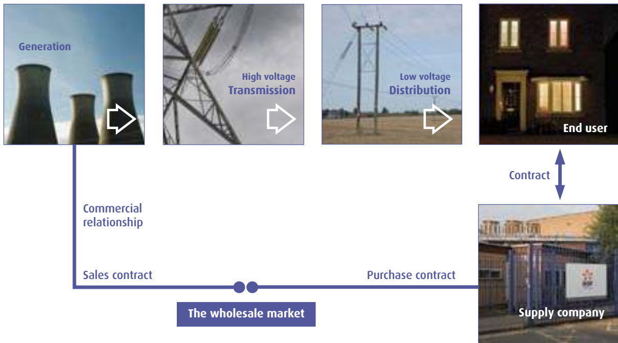
Figure 2 Technical flow of electricity
