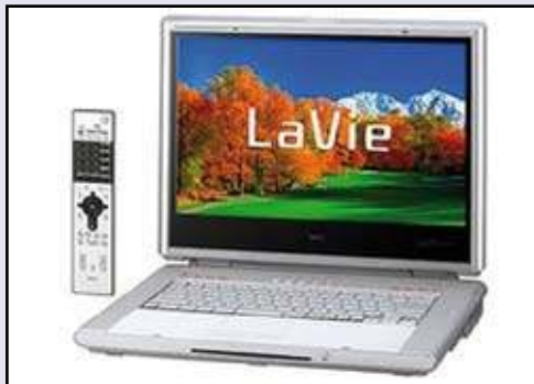
NEC LaVie T Laptop. Technology developed by NXT allows the lens screen in front of the LCD display to act as the loudspeaker.
