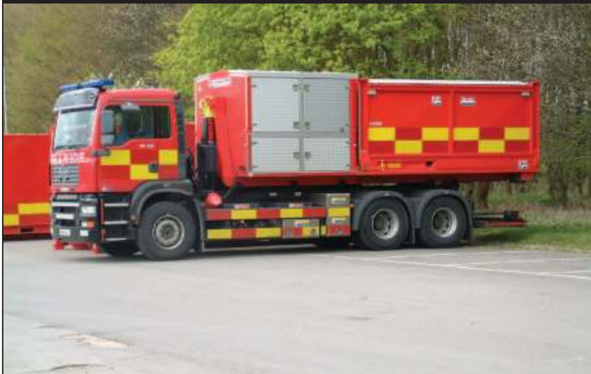
Figure 3: A High Volume Pumping Unit (19)
