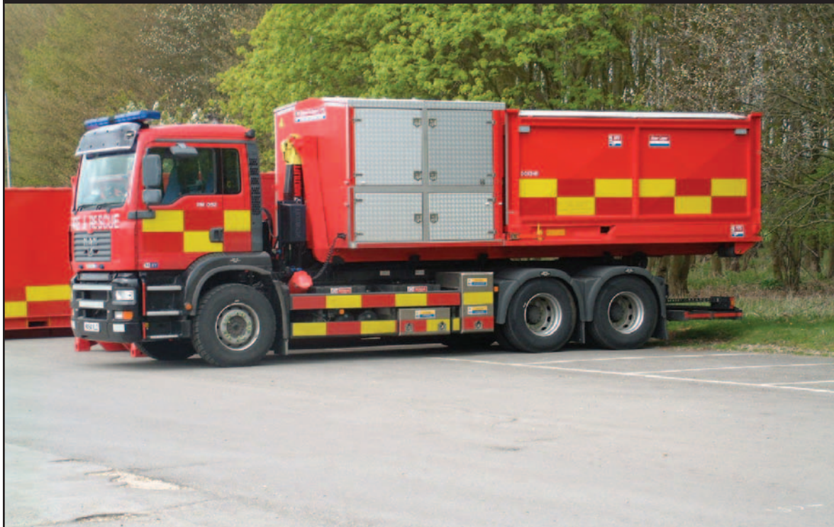
Figure 3: A High Volume Pumping Unit (19)
