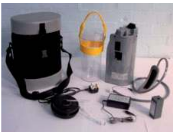
The system including container, liquid handling system and the slim-line female urinal (detailed on the right) developed by the research team for this project.
