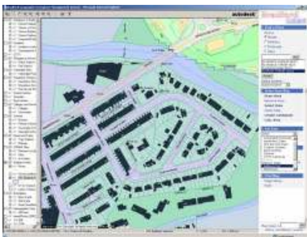
A screenshot from the Bradford MBC Geographic Emergency Management System, showing properties, facilities and infrastructure likely to be affected by a flood. On the left of the screen there is a list of other available datasets that could be added into the map (Courtesy of Bradford MBC).
