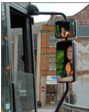
The reversing assistant should be able to see the driver in the mirrors during reversing.
